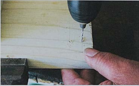
Drill out the screw holes for the block Photo by: John Webb
