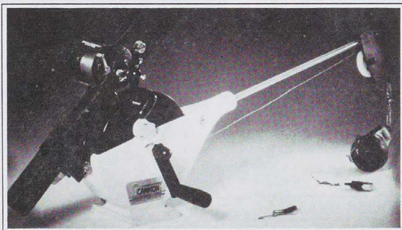
A downrigger setup showing rod and reel, the lead weight and release clip.
