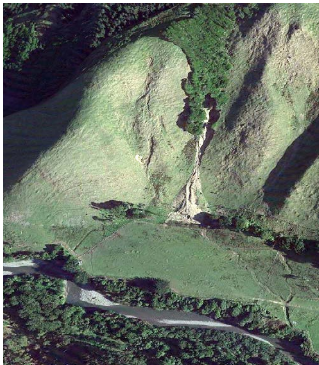
FIGURE 2-17 DEGREES OF COUPLING WITHIN FLUVIAL SYSTEMS: (A) A LANDSLIDE IN THE LOWER WAIKANAE RIVER IS MOSTLY DISCONNECTED FROM THE RIVER; THE GREAT MAJORITY OF THE LOAD IS DEPOSITED ON THE FLOODPLAIN, WITH SOME DIFFUSE FINE SEDIMENT WASHING OUT. (B) A FAN PROVIDES INTERMEDIATE STORAGE BETWEEN SITES OF ACTIVE LANDSLIDING AND DELIVERY TO THE RIVER. (C) A QUATERNARY TERRACE IN THE MID-REACHES OF THE WAIKANA RIVER SHEDS SEDIMENT DIRECTLY TO THE CHANNEL.
