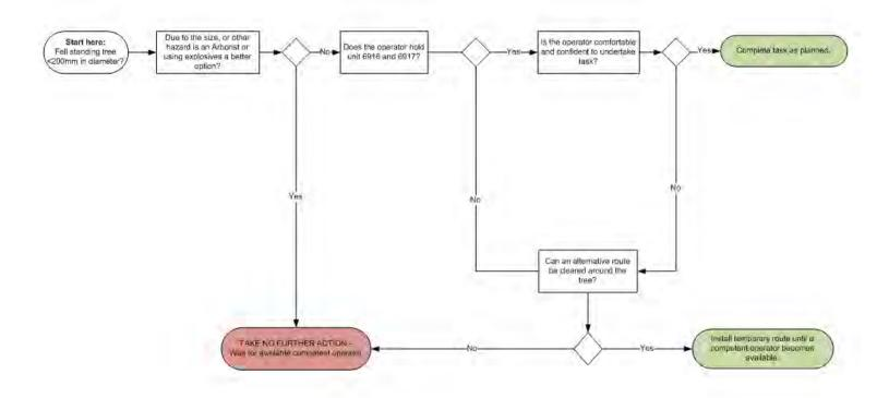
Fell a small (<200mm) live standing tree using a chainsaw v01
