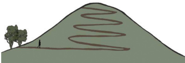
Figure 10: Poor switchback locations lead to both user and water management issues
