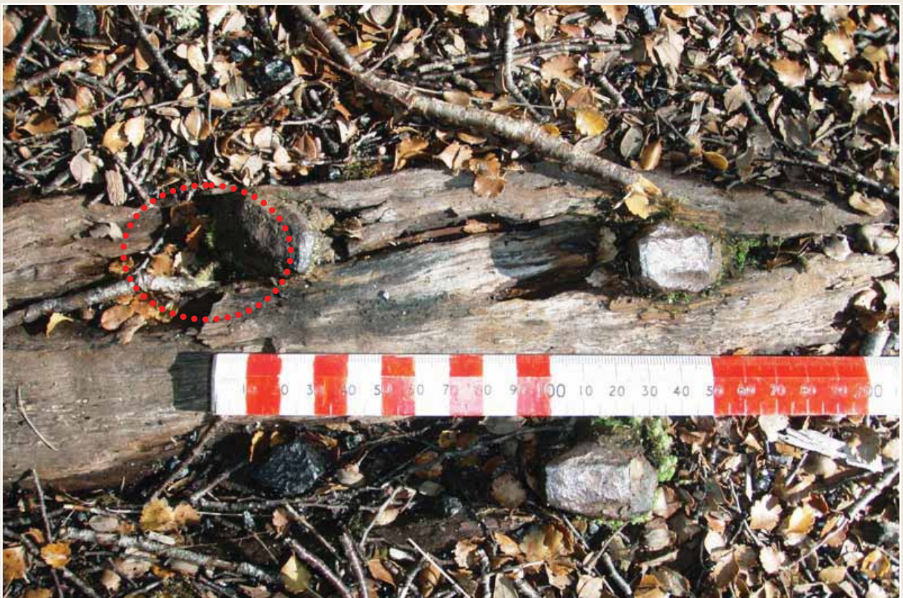
Photo 41: A set of 4 dog spikes still in the sleeper (one spike is circled).
