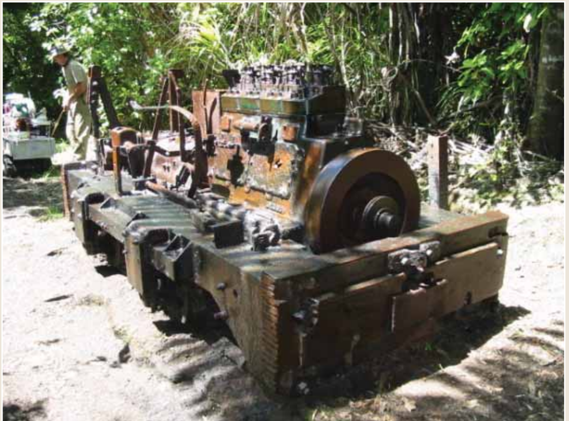
Photo 85: The remains of the Ruston and Hornsby Lokey after an application of protective oil. This lokey originally worked at the mine end of the tram.
