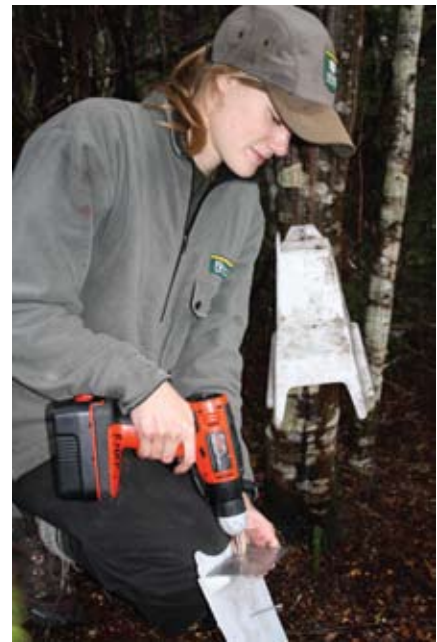
Ruth Garland, RNRP ranger, attaches an additional metal baffle to the base of a Philproof bait station.
