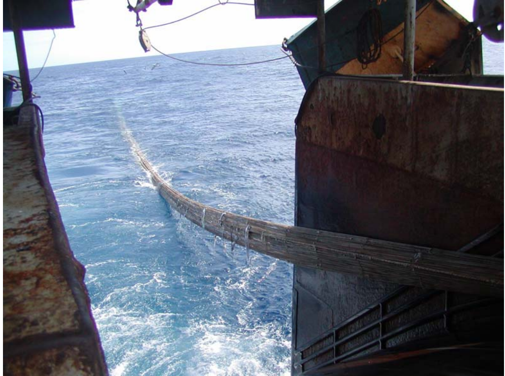
Figure 3: Retrieval of midwater trawl onto FV Aleksandr Buryachenko , with slight port helm turning the vessel to ensure net comes aboard on the port side of the trawl deck. The stern ramp quarter is acting to close the meshes by pressure on them,
