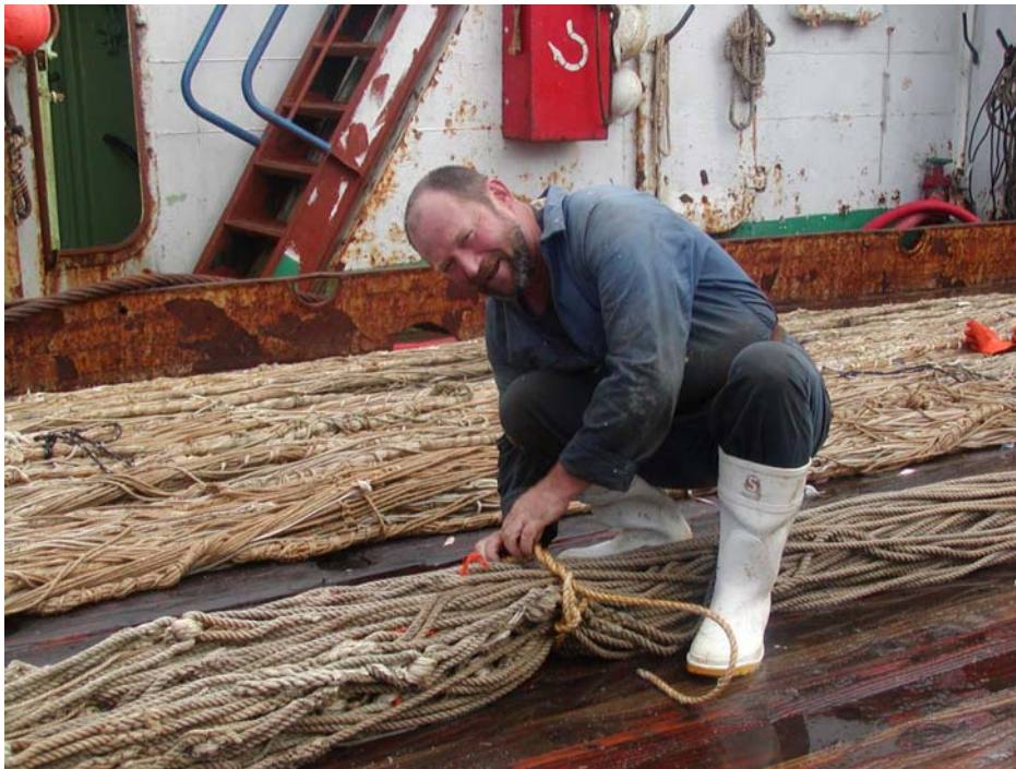
Figure 11: Trawl master Valeri net binding with 10 mm sisal rope, FV Aleksandr Buryachenko 2008
