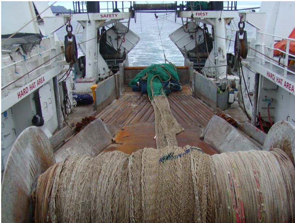
Figure 2: 28-17 Midwater trawl on the net roller and codends on deck ready to shoot, FV Taimania 2008
