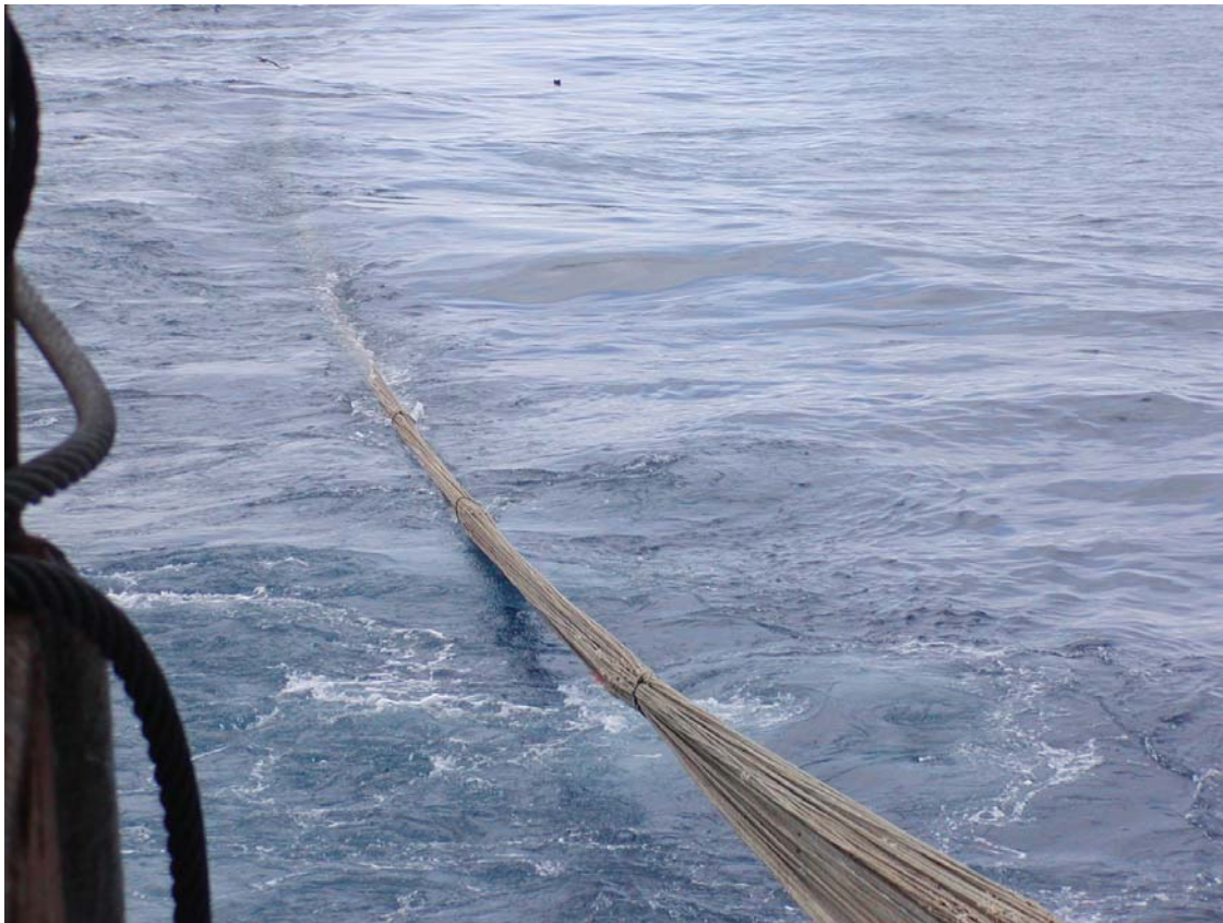
Figure 14: First three (of ten) 10 mm PPE binds on the large rope meshes holding in place at 10 m intervals, FV Aleksandr Buryachenko 2008
