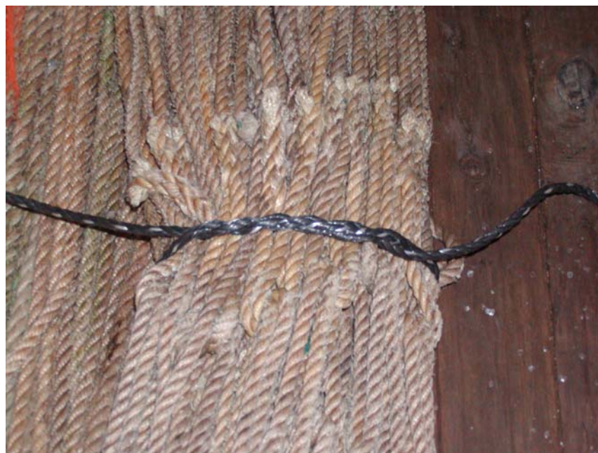
Figure 9: Reverse side of the above net bind, (following from Fig. 8) showing the three hitch slip knot which un-ties when the trawl spreads, FV Aleksandr Buryachenko 2008
