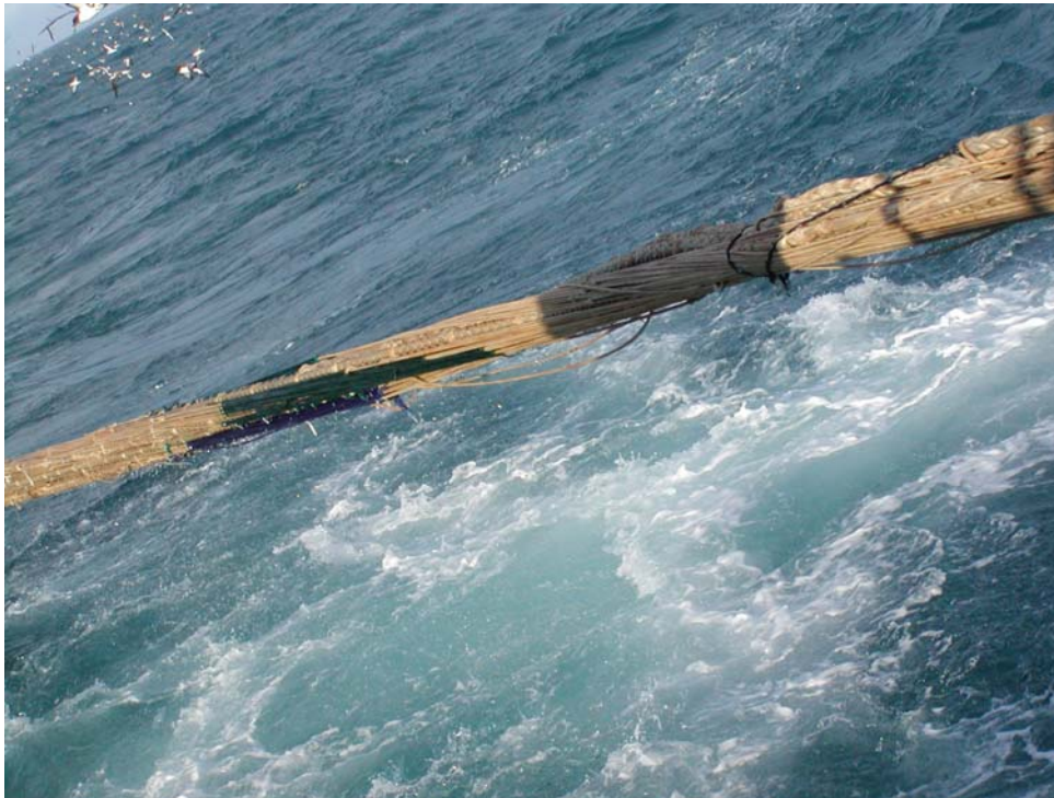
Figure 5: Trawl being hauled , net bind did not release, still tightly bound around the net at the completion of tow FV Taimania 2008
