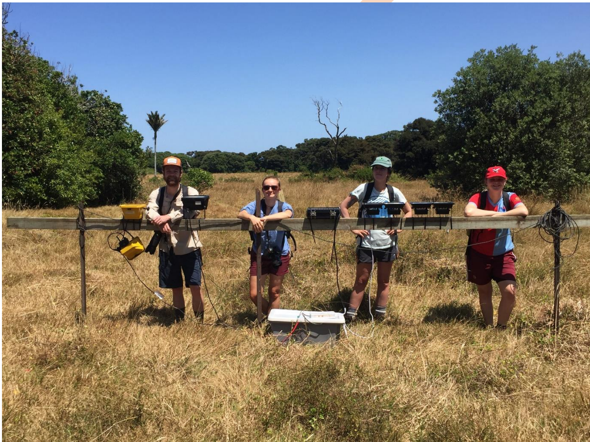
Figure 3. Light array set up on Hauturu – lights from left, halogen, fluorescent, LED flood, and LED (white, blue, green and red) . Photo: Chris Gaskin
