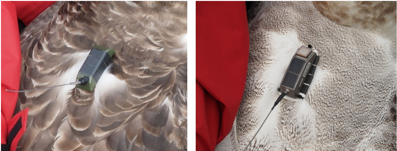
Figure 2: (left) a battery-powered TAV satellite transmitter taped directly to the back feathers of a female Antipodean wandering albatross (White-42E) and (right) a solar-powered GeoTrak satellite transmitter cable-tied to a PVC base which is taped to the back feathers of a male Antipodean wandering albatross (White-026).
