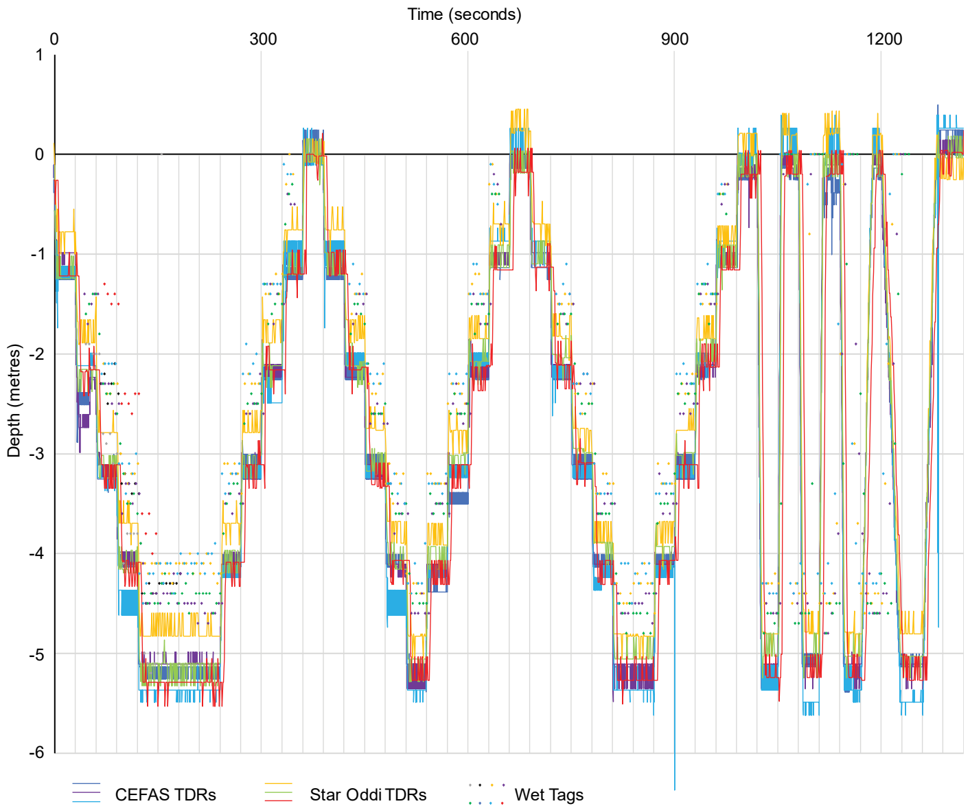
Figure 12. Plot of time vs depth for three CEFAS TDRs, three Star Oddi TDRs and eight Wet Tags deployed together in a series of controlled drops.
