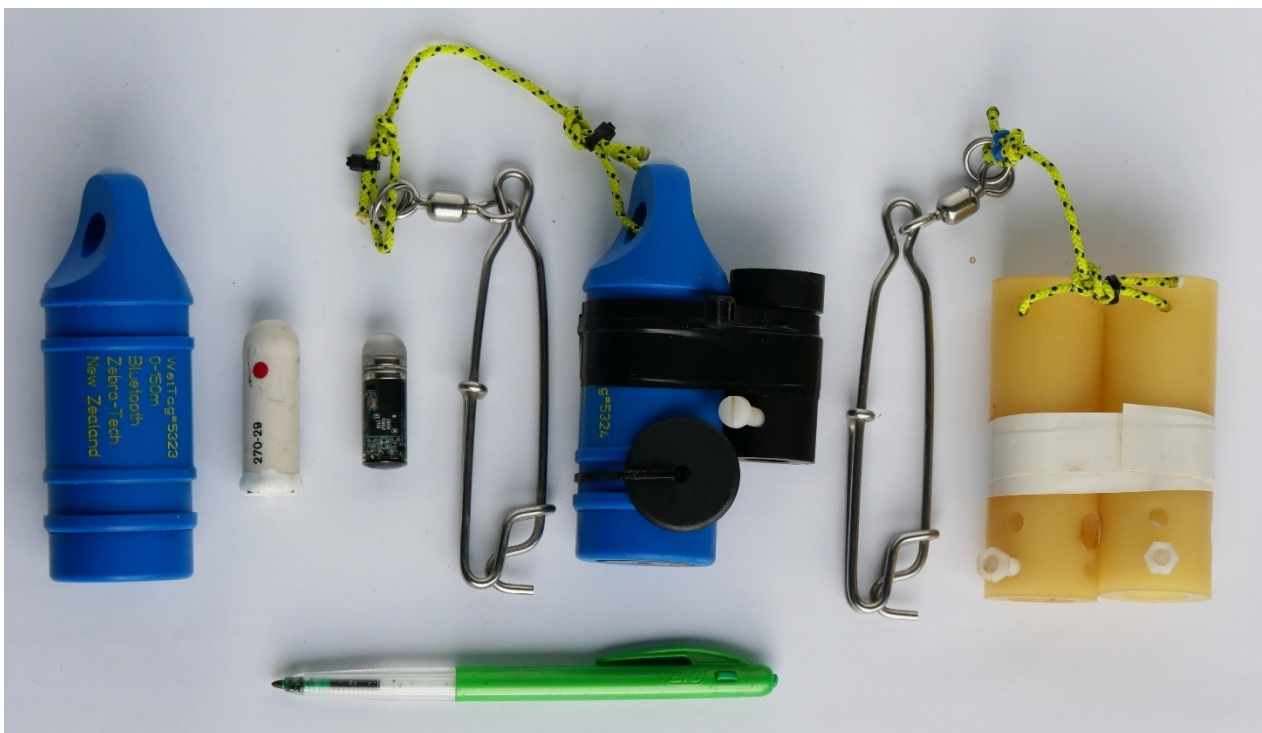
Figure 1. Photograph showing (from left to right) Wet Tag, Star Oddi TDR, CEFAS TDR, Wet tag, NFC tag, and housing for CEFAS TDR as deployed on the demersal longlines, and two Star Oddi housings used for paired deployments on the demersal longlines.
