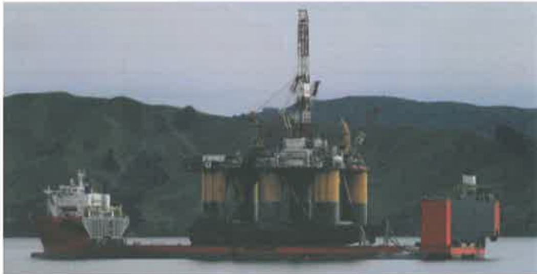
Figure 2: Kan Tan IV semi-submersible rig on vessel prior to mobilisation to the survey location.
