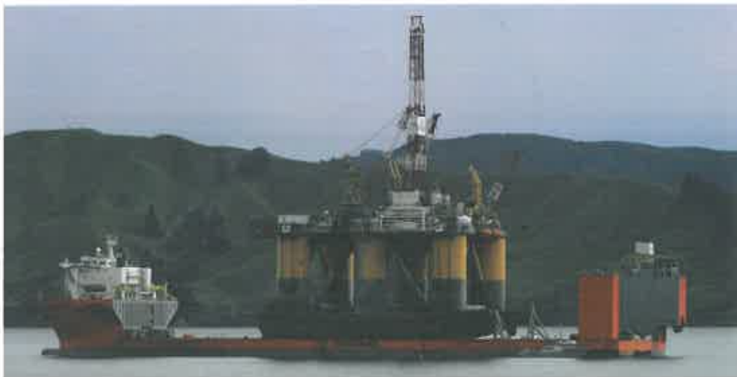
Figure 2: Kan Tan IV semi-submersible rig on heavy lift vessel in Admiralty Bay.
