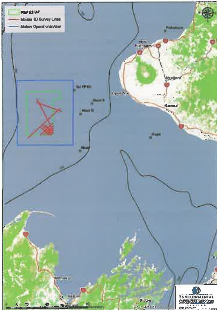
Figure 1: Location of the Mohua 2D Marine Seismic Survey with indicative survey lines.
