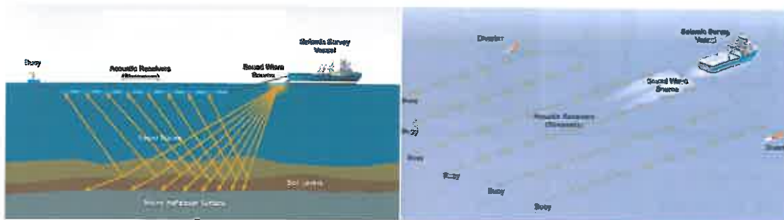
Figure 2: Schematic of a 2D MSS (left) and 3D MSS (right)
