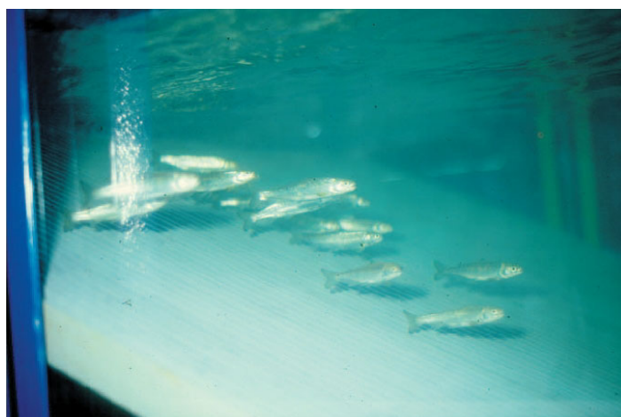
Figure 5.9: Salmon smolts remain in a position only a few centimetres before mechanical barriers - the photograph shows a 20 mm-screen arranged flat inclined to the bottom - by adjusting their swimming speed exactly to the approach velocity (ADAM et al., 1999)
