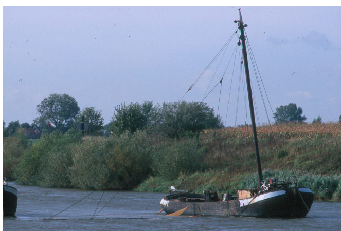
Figure 6.7: Anchored stow-net for eel in the tailwater of the hydro-power plant Lith on the Maas river (The Netherlands)
