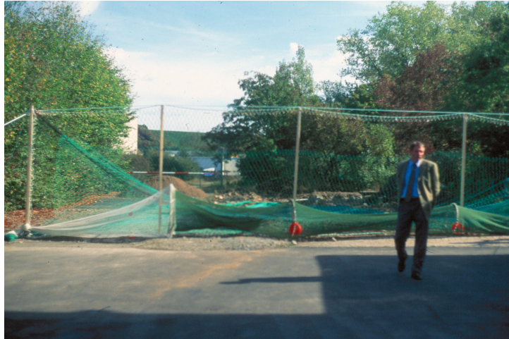
Figure 6.4: Fyke-net used for downstream migration examinations at the power plant Dettelbach on the Main river (Bavaria, Germany)
