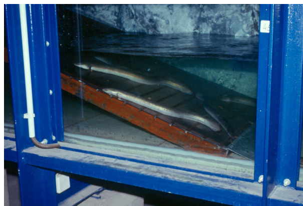
Figure 5.16: Behavioural observations on eel on a very flat inclined Wedge-Wire-Screen: the normal velocity is significantly reduced with an approach velocity of approximately 1.0 m/s. The fish will hence not be pressed against the screen, but kept away from the mechanical barrier with no risk of damage (ADAM et al., 1999)
