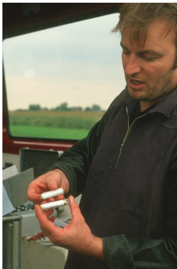
Figure 6.16: Active transponder (NEDAP TRAIL System®) for examining the downstream migration of eel in the Maas river (The Netherlands)
