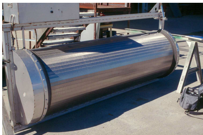
Figure 5.47: Drum screen with a diameter of 1.0 m and a Wedge-Wire-Screen surface with drive unit (workshop view, USA, Washington State)
