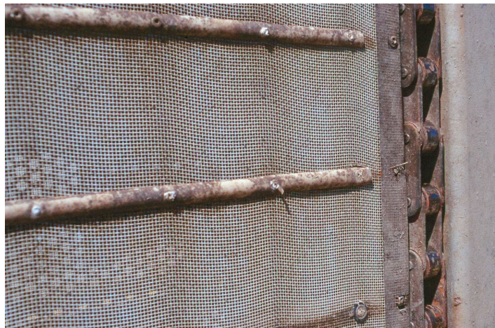
Figure 5.96: Detail of figure 5.95: Close-up view of the plastic net of 3.0 mm clear width with traverse reinforcements and driving chain
