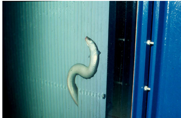
Figure 5.12: An eel that was pressed against a 20 mm-screen at an approach velocity of 0.5 m/s (laboratory examination, ARBEITSGEMEINSCHAFT GEWAESSERSANIERUNG, 1998).
