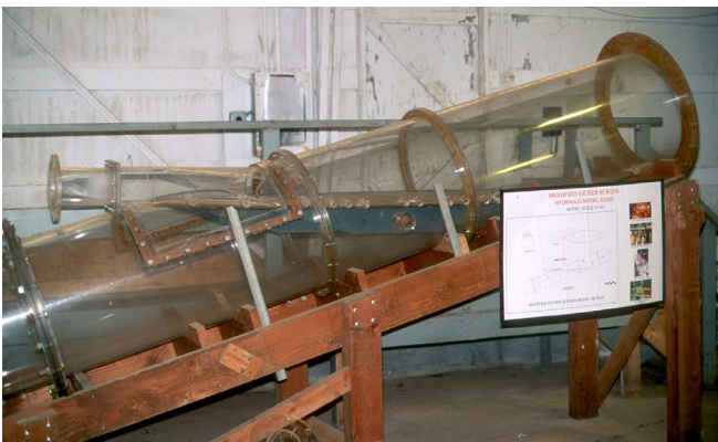
Figure 5.103: Model of the Eicher-Screen for the Elwha Dam (figure 5.105); laboratory experiment by ALDEN RESEARCH LABORATORY INCORPORATION
