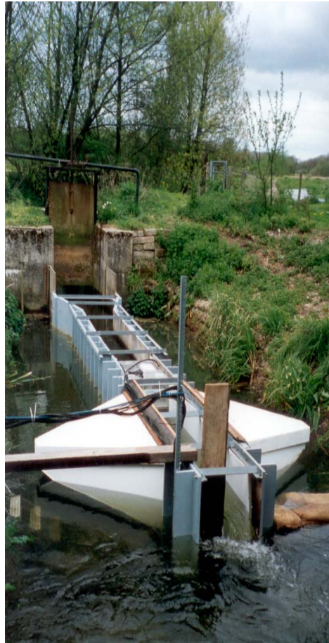
Plate 7.4 Video and resistivity smolt counting unit used to monitor smolt diverted into a bywash during BAFF™ tests conducted by the Centre for Ecology and Hydrology (CEH) at the River Frome test site in Dorset.
