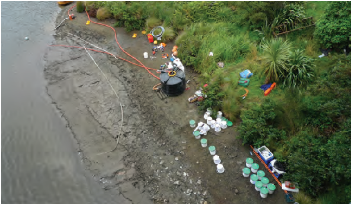
PLATE 4.2 Typical slurry mixing and tank pumping set-up used to spray rotenone onto the water surface (upper Karori Reservoir, Wellington). Green lidded buckets contain rotenone slurry as supplied from the factory.
