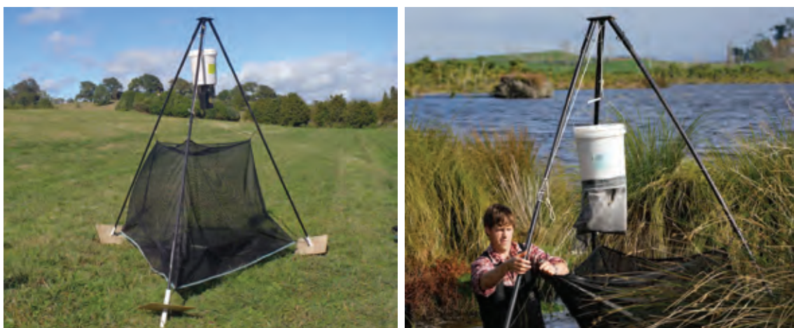
PLATE 6.2 Pod trap (left) developed by Adam Daniel (shown right) to catch koi carp, and (right) installed in Lake Ohinewai with automatic bait dispenser.
