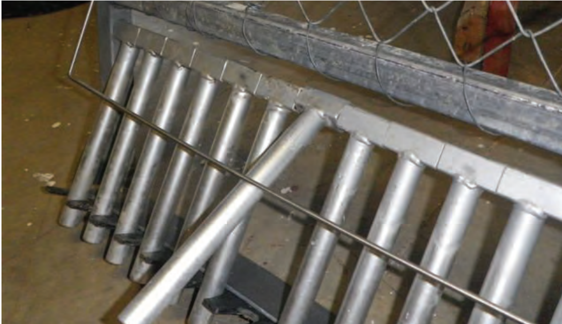
PLATE 4.5 Waikato Regional Council's 'automated' one-way finger trap based on South Australian Research and Development Institute's finger element design. When a fish pushes through any finger, a stainless bar is raised resulting in the activation of a magnetic switch that sends a signal to a telemetered box nearby. This system enables the remote monitoring of primarily invasive fish activity at a site.
