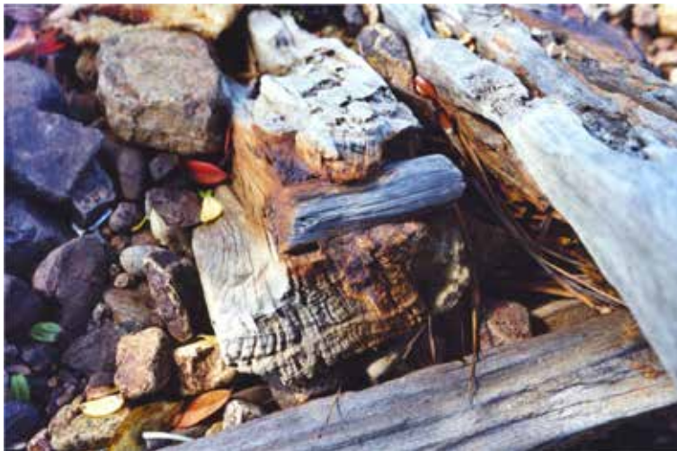
Figure 21. Detail of the rib of the Grafton hull fragment in 2002, showing the redundant treenail. Photo: Peter Petchey.
