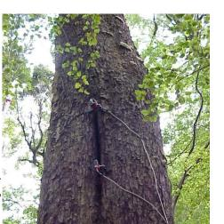
Figure 1. Single through-beam, active infrared beam counter system positioned directly outside a lesser shorttailed bat roost hole in a red beech tree.
