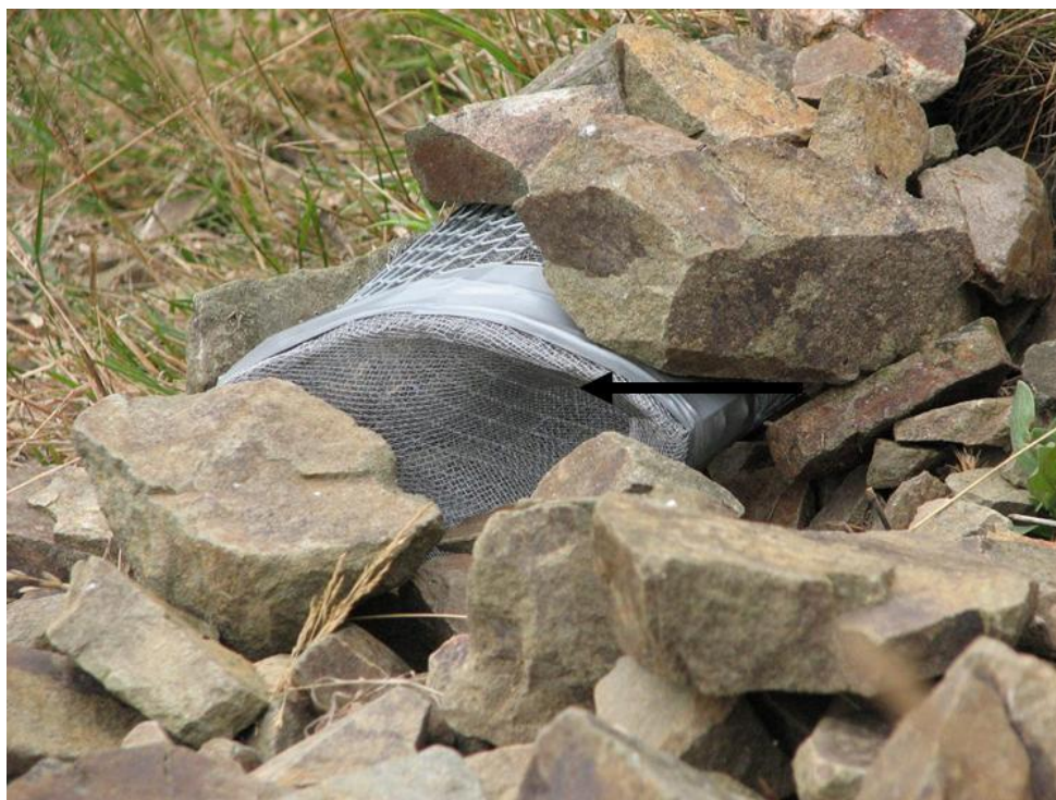
Figure 3. Single-ended funnel trap set on the edge of a greywacke scree slope. The trap is fashioned from wire mesh fly-screen and held together with wire and duct-tape. The rear of this trap (no photo available) can be opened without moving the trap, but care should be taken as lizards may dart out past the observer. The arrow points to the trap opening (photo: Konstanze Gebauer).
