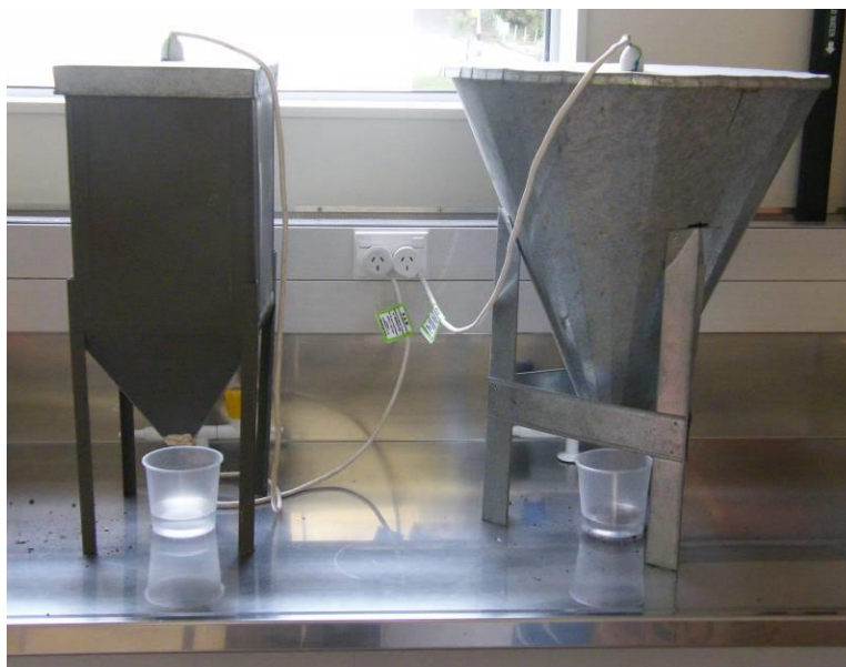
Figure 5. Two different designs of Tullgren funnel. Both have light bulbs in the lid (Figure 6) which progressively dry material suspended on coarse mesh inside (Figure 7). Invertebrates move downward as the material dries and fall into the collecting containers below.
