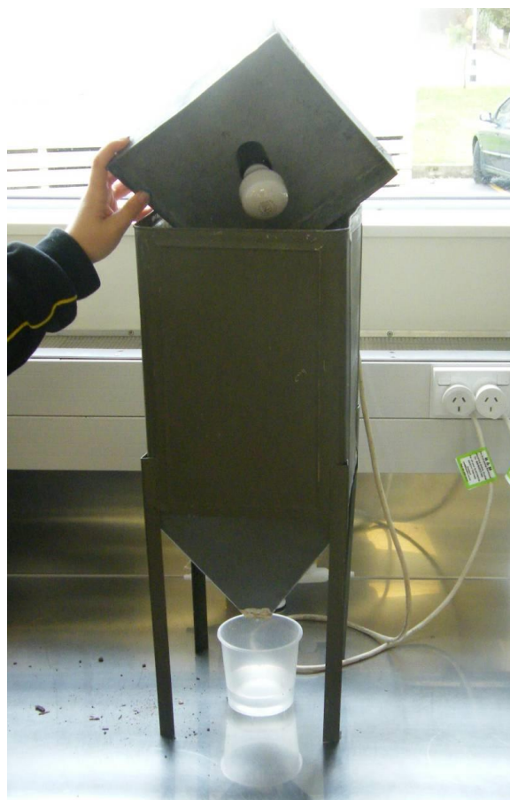
Figure 6. Tullgren funnel with lid lifted to show the lightbulb.
