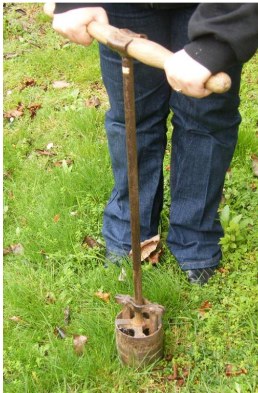
Figure 3. Soil core sampler. The handle is used to push and twist the corer into the soil. Near the base of the handle is a yoke attached to an internal disc (shown in Figure 4) which is used to push the soil sample out afterwards.
