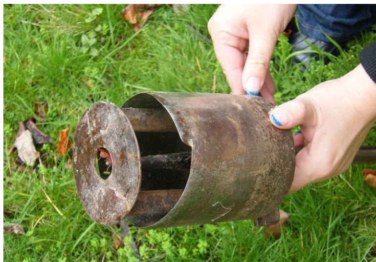
Figure 4. End of a soil core sampler. The notch in the cylinder helps dig the instrument into the soil when it is twisted while the disc (attached to the yoke shown in Figure 3) is used to push the sample out of the corer.
