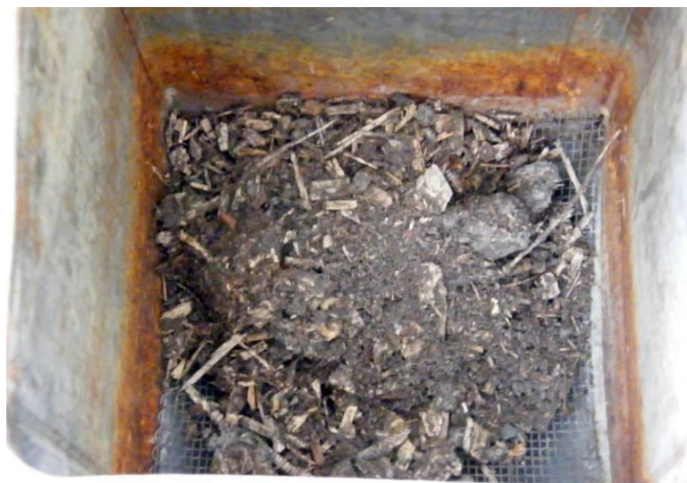
Figure 7. View inside a Tullgren funnel showing leaf litter suspended on a coarse metal mesh.
