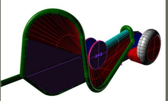
stainless steel cowling & funnel arrangement that incorporates two rollers, and which is towed behind a vessel at depth
